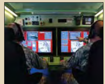
Figure 2 AAI's new Universal Ground Control Station offers a net-centric design, all-digital Tactical Common Data Link for data transmission, increased bandwidth and data security, weapons control, easy-to-read displays and up to 30 days of digitally archived data.
